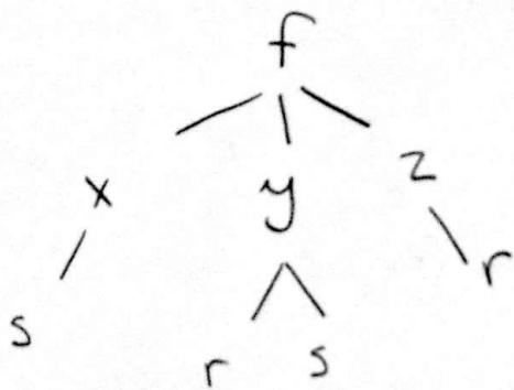
$$\frac{\partial f}{\partial s} = \frac{\partial f}{\partial x} \cdot \frac{\partial x}{\partial s} + \frac{\partial f}{\partial y} \cdot \frac{\partial y}{\partial s}$$
